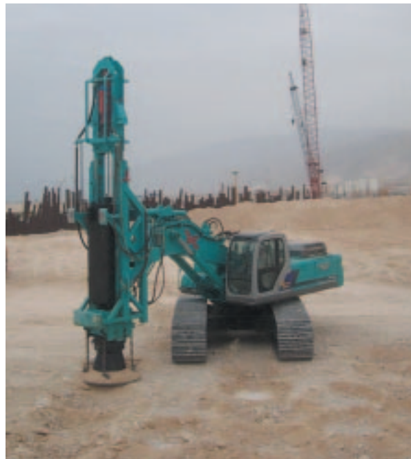
BSP Compactor, 9 tonne ram weight working in Iran
