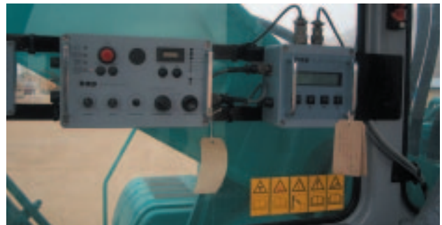
Rapid Impact Compactor controls and monitor mounted in excavator
