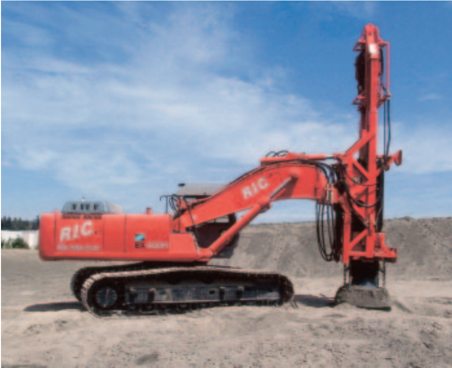
BSP Compactor, 7 tonne ram weight working in Canada
